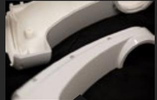
The **Cast Urethane** process produces functional plastic parts by using silicone molds and is ideal for lower quantities of molded parts.
