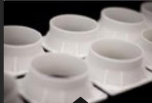
**Selective Laser Sintering** uses a high-powered CO2 laser to fuse thermoplastics, creating tough and intricate components.
