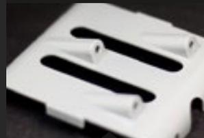
**Injection Molding** uses molten thermoplastics injected under pressure into an aluminum or steel mold creating thousands of parts.
