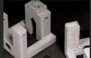
**Fused Deposition Modeling** uses a nozzle to build parts layer-by-layer by heating and extruding thermoplastic filament.
