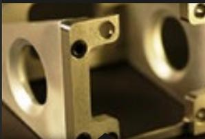
**CNC machining** is a subtractive process that removes material using computer-controlled cutters from a block or sheet.
